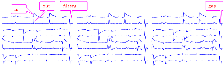
Figure 7.7: Deconvolution of leaky integrator signals with PE filters of various prediction-gap sizes. Inputs and outputs on alternate traces. Gap size increases from left to right. tsa-dleak [NR]
