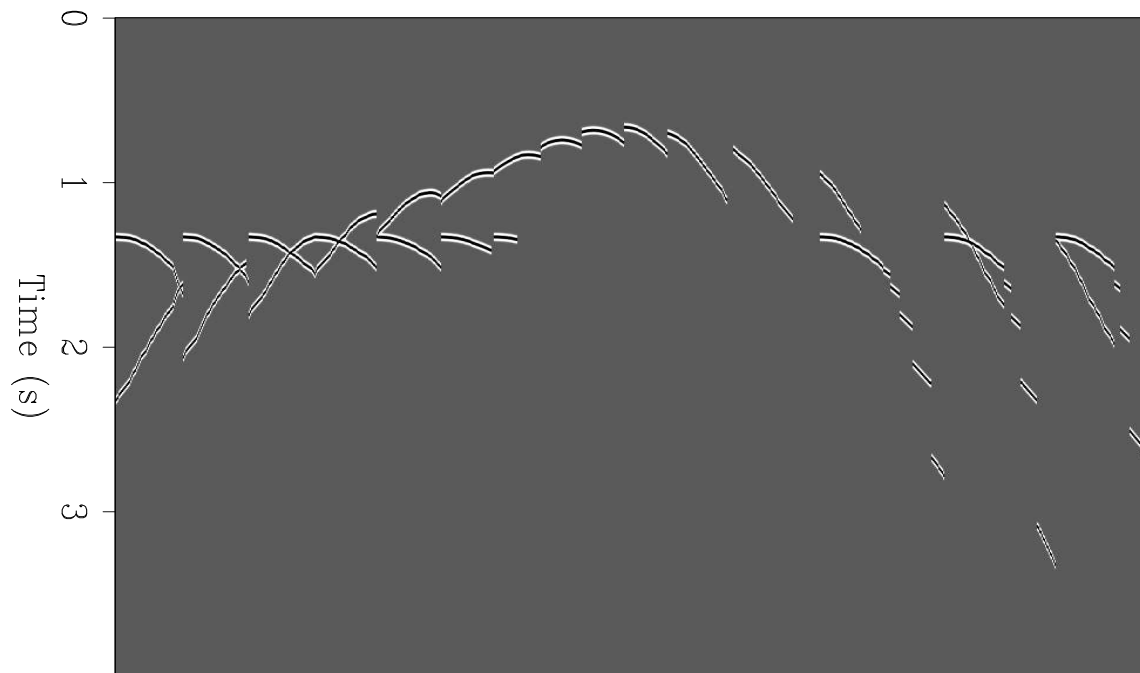
Figure 7: Synthetic shot records modeled with the proposed acquisition design. modcirc3_shots [ER]
