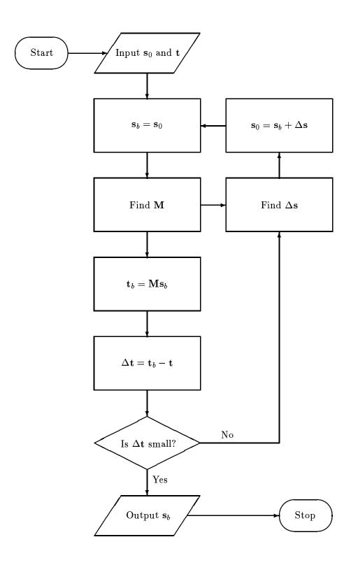
Figure 1.4: Iterative algorithm for traveltime inversion.
