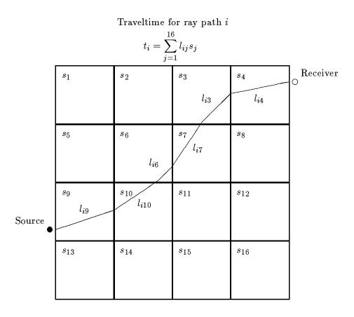
Figure 1.2: Schematic illustration of ray paths through a cell slowness model.
