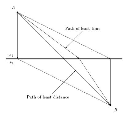
Figure 1.1: Snell's law gives the path of least traveltime from point A to point B. Other paths shown are: least distance through medium 1, least distance through medium 2, and least total distance.
