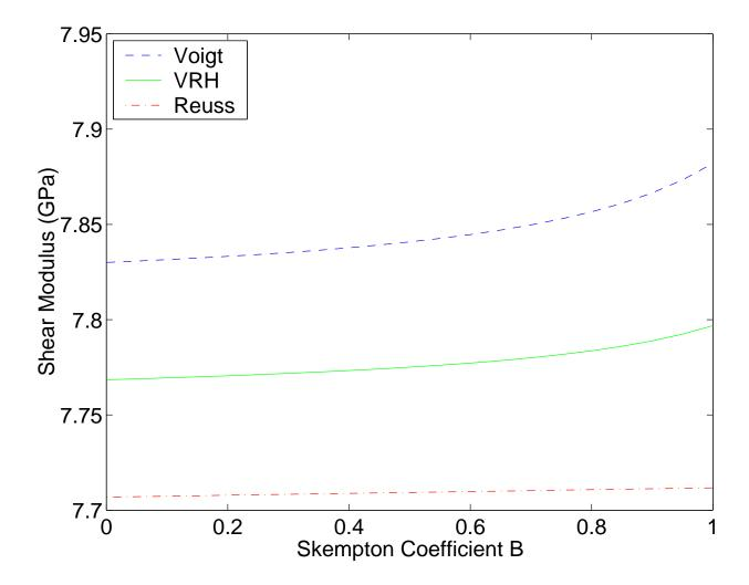
Figure 5: Example of shear modulus estimates obtained using Reuss and Voigt bounds, and the Voigt-Reuss-Hill average. Constants for the drained Trafalgar shale are given in Table 2. Other poroelastic constants are in the text.
