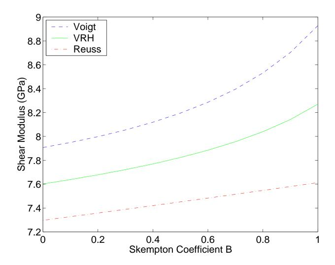
Figure 3: Example of shear modulus estimates obtained using Reuss and Voigt bounds, and the Voigt-Reuss-Hill average. Constants for the drained hexagonal (TI) medium are given in Table 1. Other poroelastic constants are in the text.
