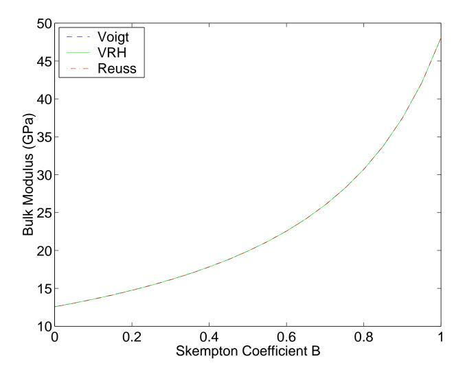
Figure 4: Example of bulk modulus estimates obtained using Reuss and Voigt bounds, and the Voigt-Reuss-Hill average. Constants for the drained Trafalgar shale are given in Table 2. This figure provides further graphical confirmation of the optimality<sup>44</sup> of the Voigt and Reuss bounds since they are very close over the entire range plotted here.
