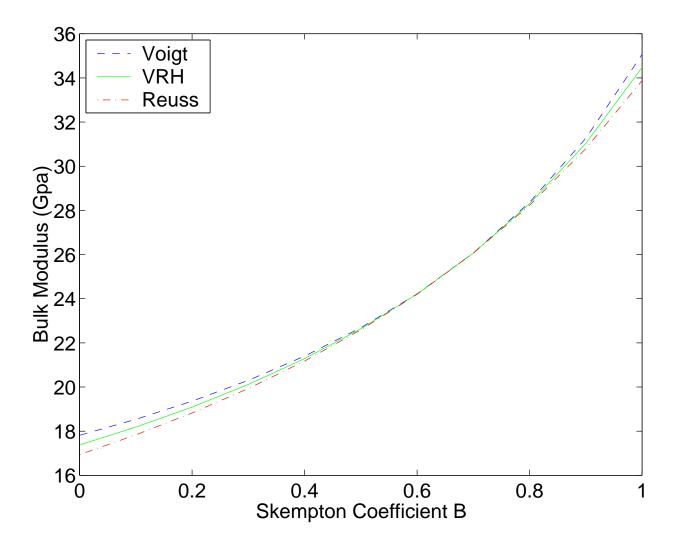
Figure 2: Example of bulk modulus estimates obtained using Reuss and Voigt bounds, and the Voigt-Reuss-Hill average. Constants for the drained hexagonal (TI) medium are given in Table 1. Note that this figure provides graphical confirmation of the optimality<sup>44</sup> of the Voigt and Reuss bounds since they nearly meet here at about B = 0.7.
