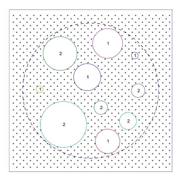
Figure 1: Schematic diagram for the coherent potential approximation (CPA) concept. The true composite is replaced by a large sphere (dashed circle) containing spherical inclusions of type-1 and type-2 constituents in the proper relative proportions. The matrix (type-\*) is composed of a material with adjustable elastic constants. When the adjustments have been made so there is no net scattering, the composite and the surrounding matrix presumably have the same effective properties.
