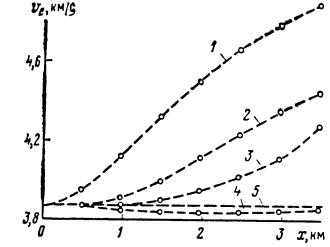
FIG. 2. Test results. This figure is reproduced from Malovichko (1979). It shows measured vertical-raypath rms velocity (vertical axis) versus total spread length (horizontal axis). Each curve represents a different measurement technique; see the text for details.
