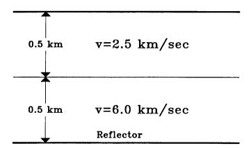
FIG. 1. Test model. This is the model used by Malovichko to produce the results in Figure 2. Note the large velocity contrast.
