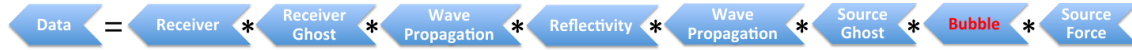
Figure 1: The convolutional model of seismic data. The purpose of the seismic method is to estimate the reflectivity. All other physical filters must be accounted for. In this paper we focus on deterministic methods for debubbling. [NR] joseph1/. chart
