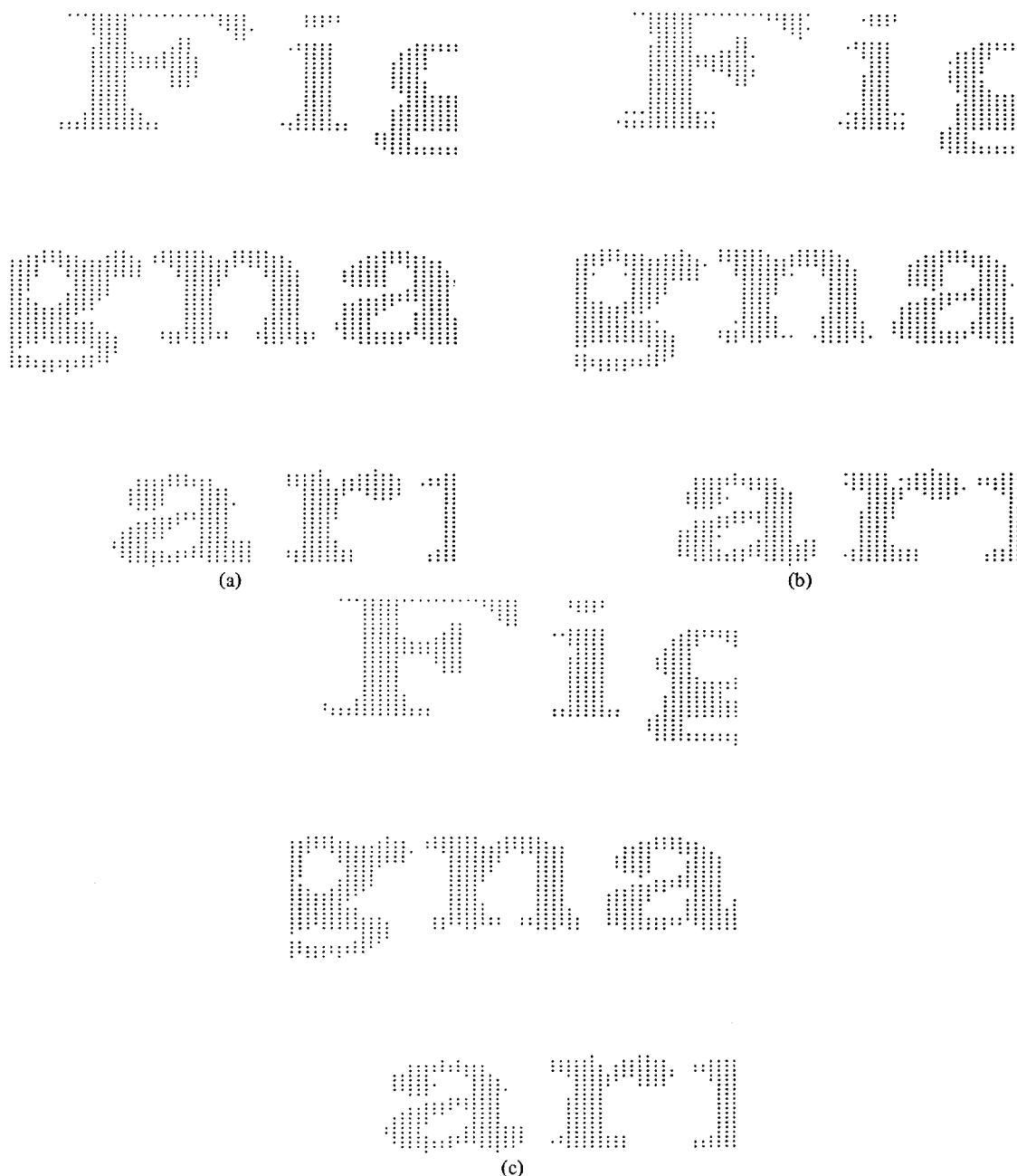
Fig. 12. 0.647 reduction of Figs. 9 and 10 by truncated sinc function interpolation. (a) Using Fig. 13(a). (b) Using Fig. 13(b). (c) Using Fig. 13(c).
