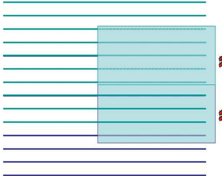
Figure 2: Schematic of fold coverage of two adjacent sail lines. gabriel2-sketch2 [NR]
