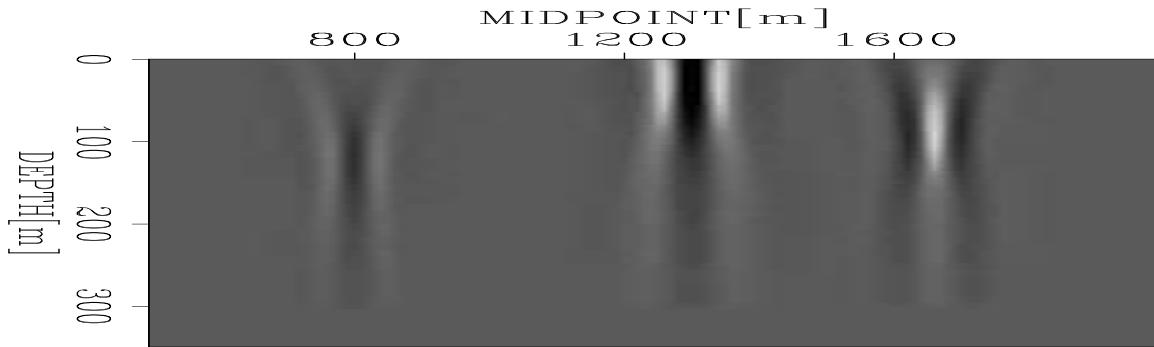
Figure 4: Slowness backprojection of the image perturbation using one nonlinear WEMVA iteration, with an unregularized solver. nick1-slow_proj [CR]
