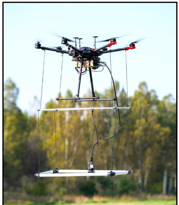
Geonics EM61 Lite suspended from a DJI Matrice 600 Pro UAS
