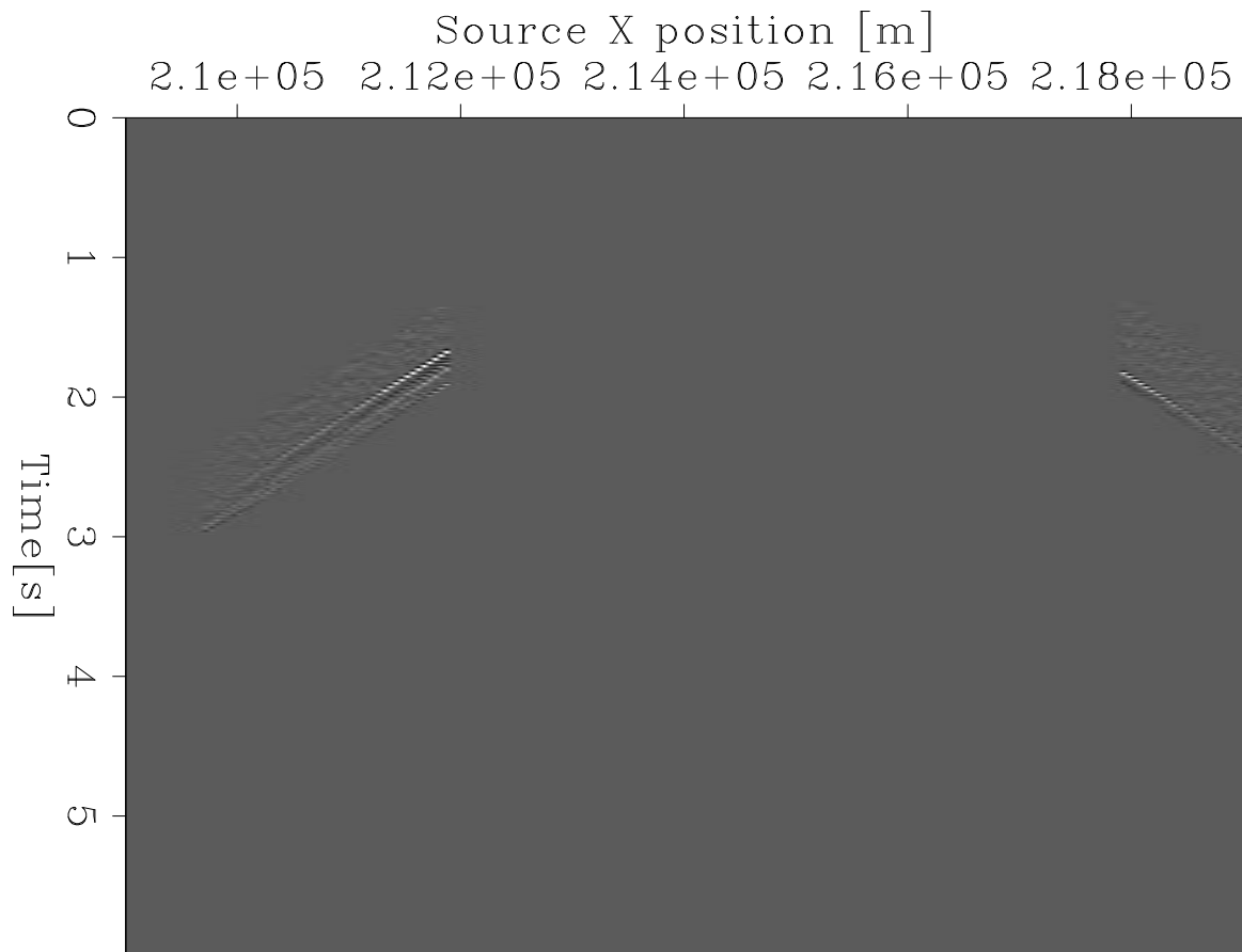
Figure 3: Hydrophone data window (isolating the refraction events) used for estimating PZ-summation filter. [CR]
