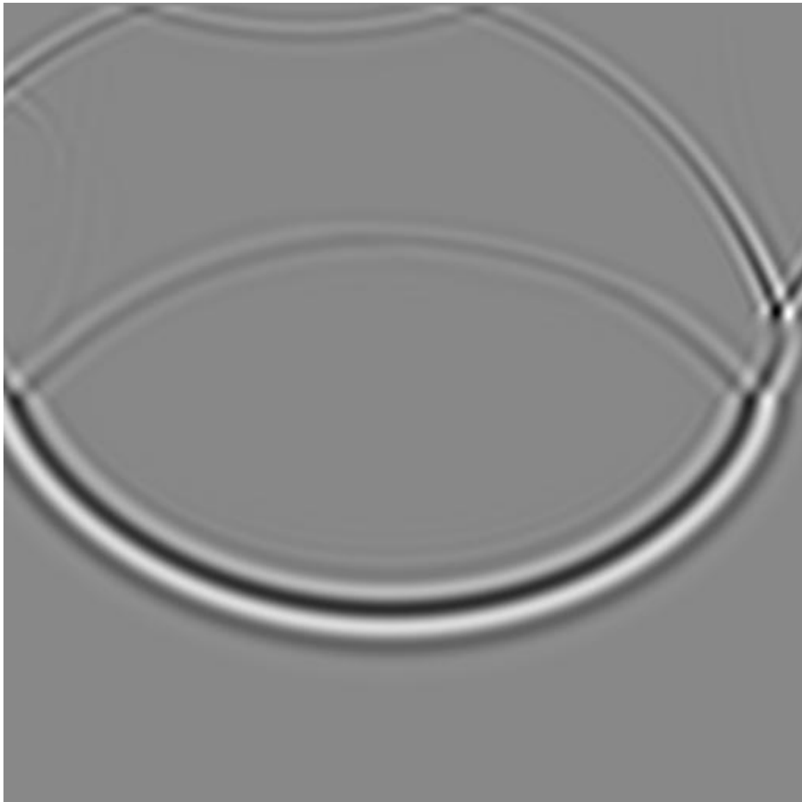
Figure 2: Snapshot of the wavefield captured from the CM FrameBuffer. Notice the absorbing boundary conditions on the sides and the free surface at the top.
