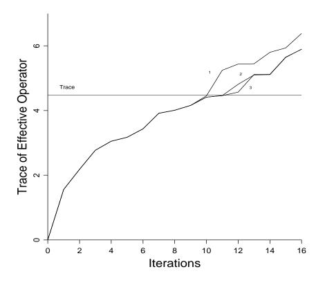
Figure 9: LSQR with partial reorthogonalization – using both first and last one, two, or three. resol-sum311 [NR]
