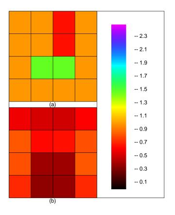
Figure 1: Target model slowness (a) and resolution (b) for truncated SVD using 10 largest eigenvalues. resol-casea [NR]
