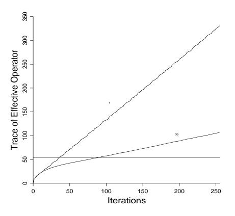
Figure 11: LSQR with partial reorthogonalization – using first or first 35 vectors. resol-ex3510 [NR]
