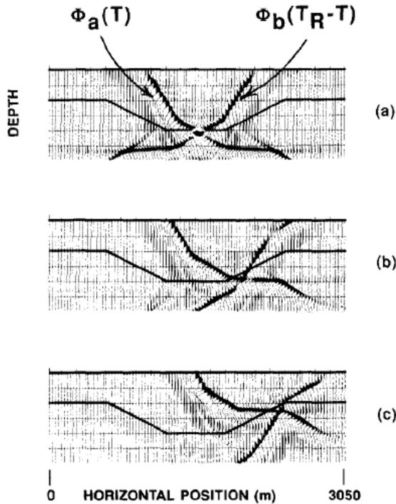
FIG. 5. Wavefronts obtained by downward continuation of the arrivals in Figure 4. The sum of the time instants of the wavefronts in each frame is equal to the reciprocal time. Frames a, b, and c correspond to  $t = 0.5 t_r$ ,  $t = 0.6 t_r$ , and  $t = 0.7 t_r$ . The wavefronts always cross on the refractor boundary.
