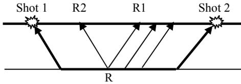
The total refraction traveltime from Shot 1 to Shot 2 is  $T_R$ . We want to derive a reflection wavefield with a path from R2 to R and then R1, converting R2 to a source point. If we denote this reflection traveltime as  $T_{rfl}$ , then:
