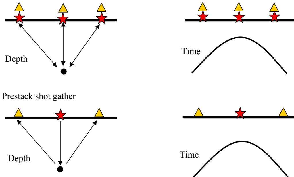
**Time Migration:** collapse hyperbola to a reflection point in time by using RMS velocity
