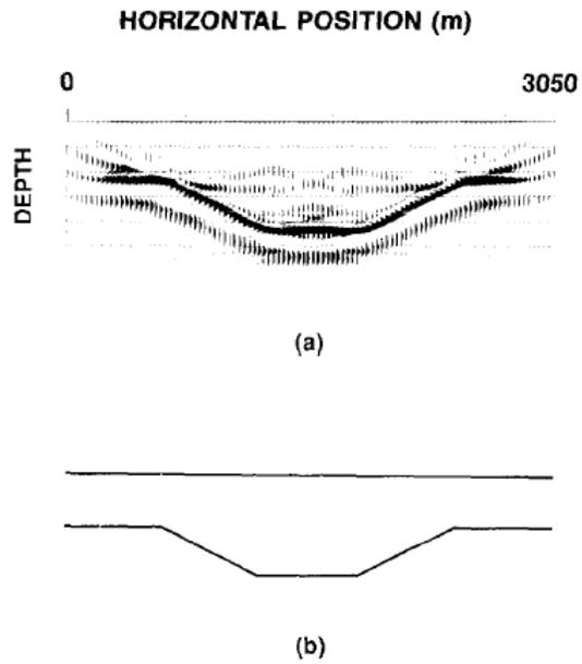
FIG. 6. (a) Image of the refracting interface obtained by downward continuation of the refracted arrivals of the forward and reversed gathers. (b) The original model.
