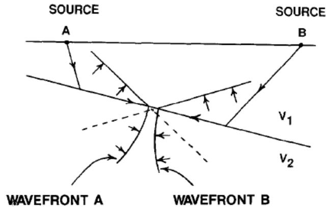
FIG. 1. Wavefronts for reversed refraction profiles. The unrefracted wavefronts (dashed line extensions) cross on the refractor boundary when  $t_a + t_b = t_r$ , where  $t_r$  is the traveltime from source A (source B), along the refractor, to detector B (detector A).
