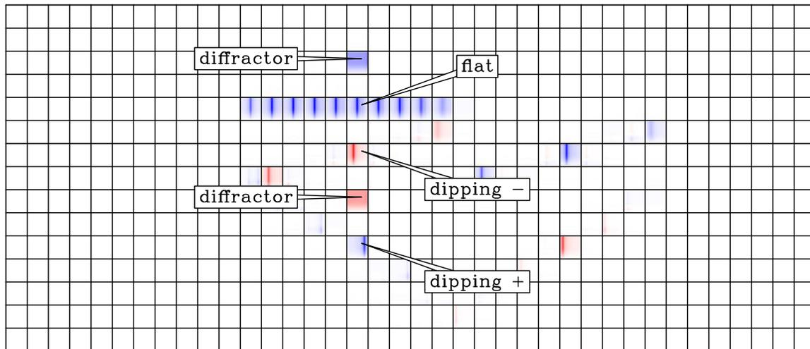
Figure 6: Multi-angle decomposition for the image in Figure 5. In each box, the horizontal axis corresponds to the dip angle  $\alpha$ , and the vertical axis corresponds to the scattering angle  $\gamma$ . `paul3-chck1` [CR]
