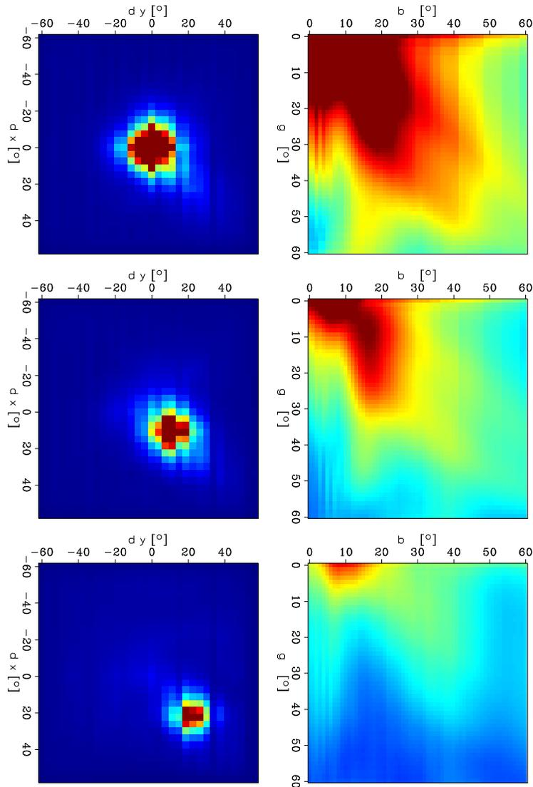
Figure 11: 3-D multi-angle decomposition of migrated images. On the left, the panels correspond to summation over the scattering  $\gamma$  and azimuth  $\beta$  angles. On the right, the panels correspond to summation over the projections of the normal to the reflector,  $\delta_x$  and  $\delta_y$ . From top to bottom, each pair of panels corresponds to different depths  $z = 1000, 1150, 1380$  at the same location in the image  $m_x = 1000, m_y = 800$ . `paul3-slic3d` [CR]
