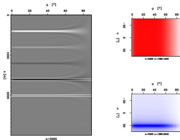
The next example corresponds to a 3-D seismic image (Figure 9) obtained by narrow-azimuth migration (Biondi, 2003). The figure depicts the zero offset  $h_x = 0, h_y = 0$  image, although in reality the cube has the full 5 dimensions of 3-D prestack data.
