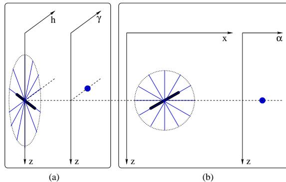
Figure 3: A sketch of a generic reflection experiment and its associated angle decomposition. The left panel corresponds to the  $x - z$  location of the reflection point in the image. In the 2-D case, at every point in image, the reflectivity is described by two angles,  $\alpha$  and  $\gamma$ . paul3-mag [NR]
