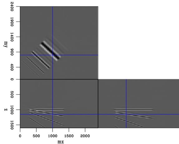
Figure 10: Angle gather obtained by the traditional ADCIG equation (left). 3-D angle gather obtained by summation over the reflector dip angles  $\delta_x$ ,  $\delta_y$  and acquisition azimuth  $\beta$  (right).
