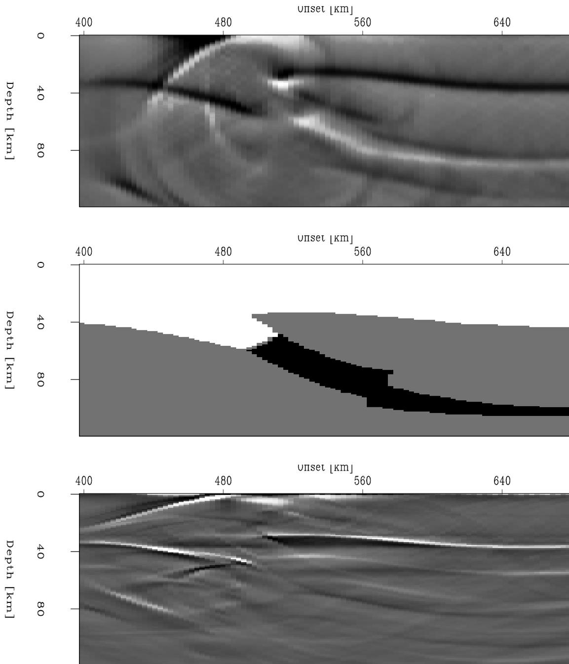
Figure 3: a) Forward-scattered P-S mode image; b) Synthetic Model; c) Backscattered P-P mode image. jeff2-fsbs [CR]
