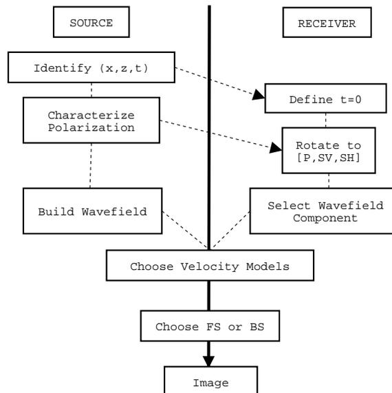
After identifying source parameters, time zero and the total length of the record to be migrated is determined. Three-component receiver arrays are necessary to exploit the full range of wavefield scattering combinations in these experiments. With the introduction of vector displacements, a rotation of data components is defined that maps energy from the recording geometry  $[Z, N, E]$  to an alignment with source wave vector axes  $[P, SV, SH]$ .
