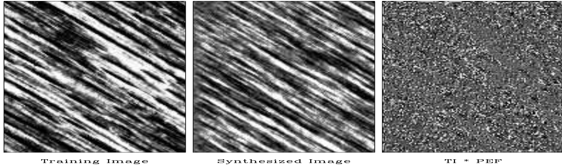
Figure 6.4: Synthetic wood grain has too little white. This is because of the nonsymmetric brightness histogram of natural wood. Again, the PEF output looks random as expected. mda-wood [ER]
