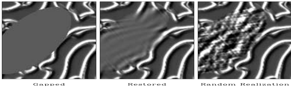
Figure 6.18: The theoretical model is a poor fit to the ridge data since the prediction must try to match ridges of all possible orientations. This data requires a broader theory which incorporates the possibility of nonstationarity (space variable slope). mda-ridges-hole-fillr [ER,M]
