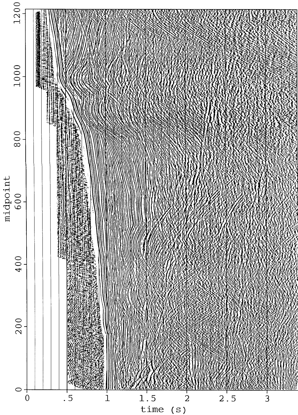
FIG. 6. Stacked section. This section has been created by interpolation between constant velocity sections using the velocity function shown in figure 4.
