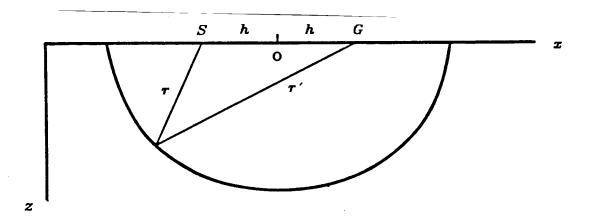
FIG. 1. An elliptical reflecting boundary surrounding a constant velocity region. The source is placed at the focus labelled S and the geophone at focus G. The distance from a boundary point to the source is denoted by r and to the geophone by r. The origin for Cartesian coordinates is placed midway between the source and geophone.
