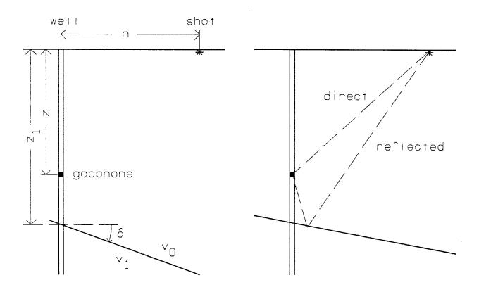
FIG. 2. (a) Geometry of an offset VSP (b) Ray paths for direct and reflected arrivals
