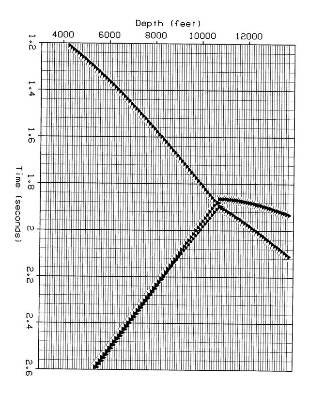
FIG. 5. Model 2:  $v_0$ =6750 ft/s,  $v_{1p}$ =17500 ft/s,  $v_{1s}$ =10000 ft/s
