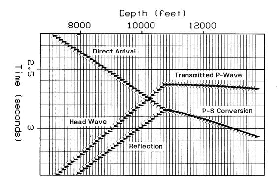
FIG. 4. Model 1:  $v_0$ =4500 ft/s,  $v_{1p}$ =24000 ft/s,  $v_{1s}$ =8000 ft/s
