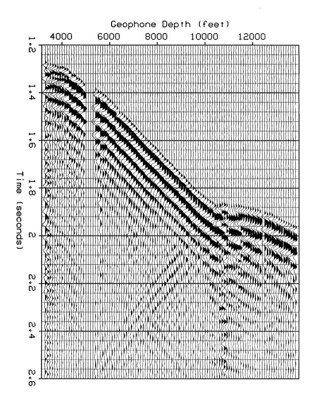
FIG. 1. Example of offset VSP data (courtesy of Amoco and Western Geophysical). The shot in this example was offset 7000 feet from the well.
