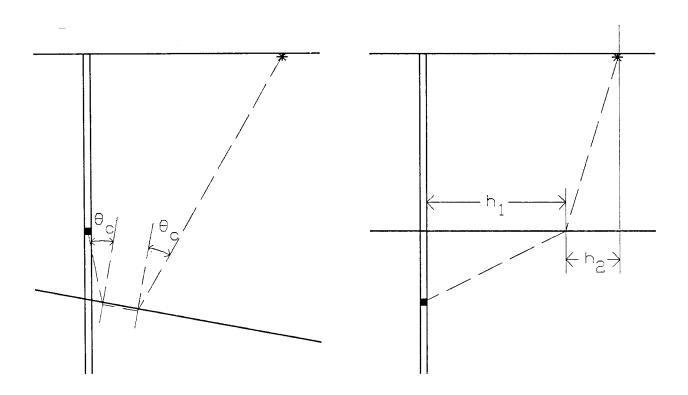
FIG. 3. (a) Ray path for a head wave (b) Ray path for transmitted or converted arrivals.
