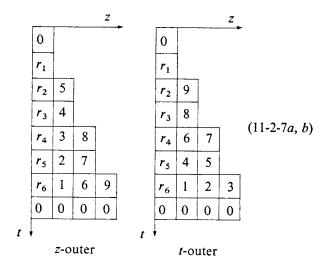
FIG. 1.. Schematic z-outer and t-outer 15° migrations. Both advance the stacked time section,  $r_i$ , to the same migrated, diagonal section in the indicated orders. Figure reproduced from Claerbout (1976).
