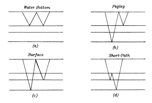
FIG. (0.1). Raypaths are displayed for (a) water-bottom multiple, (b) pegleg multiple, (c) general surface multiple, and (d) short-path multiple.
