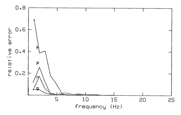
FIG. 1. Relative error versus temporal frequency for a downward continuation problem. Only the first 26 frequencies after DC are plotted. Zero frequency is the blank at the left margin. For curve (h), the linear equation solver was Householder elimination. For curve (p), the subroutine pentc from SEP-26. Curve (n) was generated by a Gaussian elimination routine with the pivoting option turned off. Curve (g) is the result of employing Gaussian elimination with partial pivoting.
