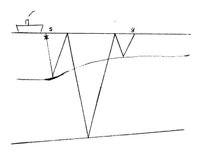
FIG. 1. Water depth and seafloor reflectivity are functions of shot and geophone location. The Backus operator makes no allowance for this.
