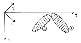
FIG. 3. The correlation between upcoming and downgoing wavefields at the seafloor is removed from the upcoming wave for each common geophone location (1). Residual correlation common to shot locations is then removed (2).
