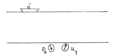
FIG. 2a. Objective wavefield consists of downgoing shot and upcoming receiver both below the seafloor.
