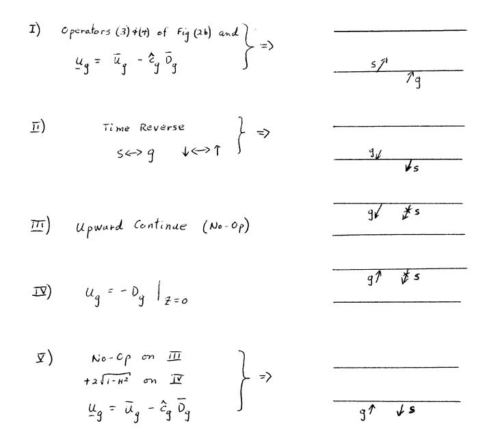
FIG. (2c). Conceptual steps in the 0-dip algorithm.
