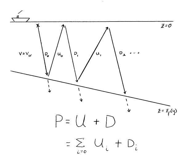
FIG. (A1). Decomposition of upcoming and downgoing pressure field in water layer.
