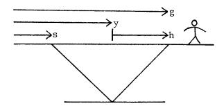
FIG. 2. Conventional reflection seismology geometry.
