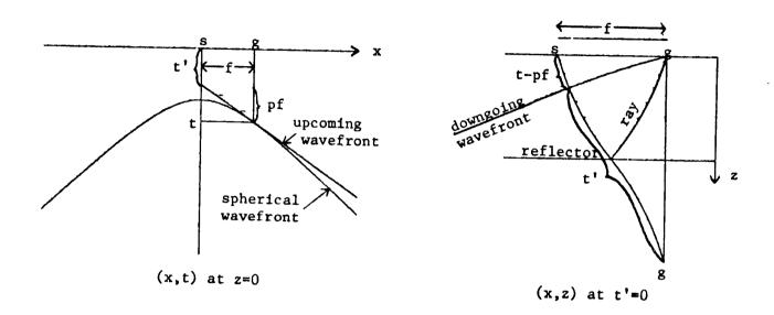
FIGURE 1.—An arbitrary stepout p (slope in x-t plane) is chosen tangent to a hyperbolic arrival. When projected back to zero offset the traveltime t' is exactly that for the downgoing wavefront in the figure to travel down the ray to the reflector and back up to the surface geophone at g.
