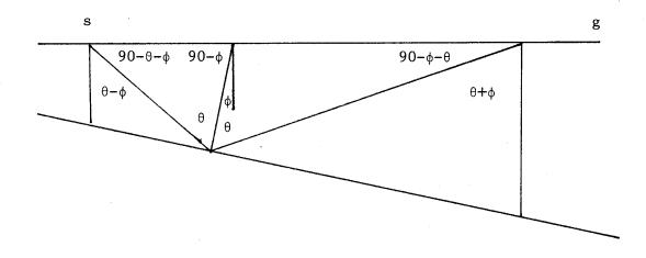
First check that the sums of the interior angles of the triangles are all 180 degrees. Then we have the trigonometric identities
