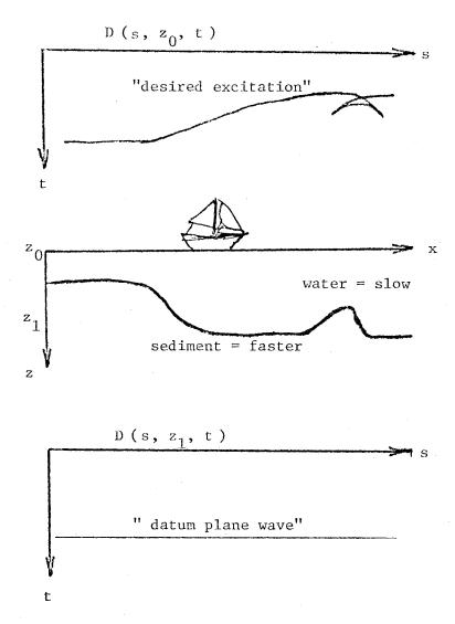
Figure 4.8. In order to achieve a downgoing plane wave at the datum depth  $z_1$ , another wave "desired excitation" must be initiated at  $z_0$ . The "desired excitation" may be computed by projecting the "datum plane wave" up through the sea floor topography.
