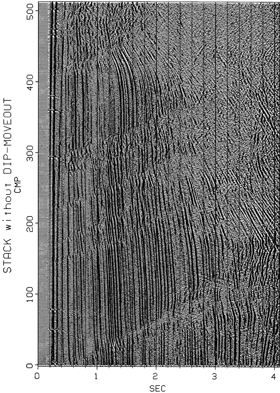
FIG. 1.10b. CMP stack of NMO-corrected data. DMO was not applied in computing this section. This stack was migrated to obtain the section plotted in Figure 1.8b. Compare this section with that of Figure 1.10a to verify that omitting DMO from the processing sequence degrades the dip bandwidth of the CMP stack. The CMP interval is 0.033 km.
