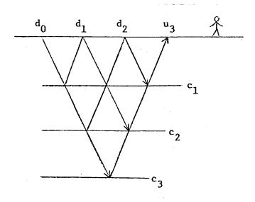
FIG. 1. Ray-path geometry for upcoming wave  $u_t$  at the surface at time t=3 in terms of waves  $d_t$  downgoing from the surface at earlier times and reflection coefficients  $c_t$  at uniformly spaced traveltime depths.
