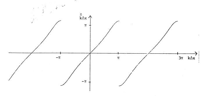
FIG. 3. Accuracy of the second-derivative representation of (7) as a function of spatial wavenumber. The sign of the square root of (7b) was chosen to agree with k in the range  $-\pi$  to  $\pi$  and to be periodic outside the range. (Curve computed by Dave Hale.)
