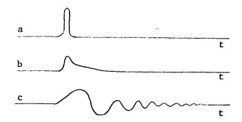
FIG. 1. (a) A pulse. (b) A pulse slightly dispersed as by the physical dissipation of high frequencies. (c) A pulse with a substantial amount of frequency dispersion, as could result from data processing.
