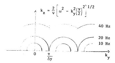
FIG. 2. The effective dispersion relation of the wave equation when the hor-zontal axis is sampled. Values are given for zero-offset migration where  $\Delta y = 25$  meters and velocity v = 2000 m/sec. The semicircular arcs correspond to frequencies of 40, 20, and 10 Hz.
