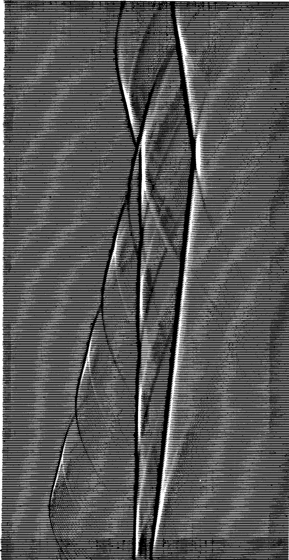
FIG. 6.10. Same results as in figure 6.3, but in order to more realistically simulate the bandwidth of real data the traces have been differentiated with respect to time. The broadening of the waveform, caused by anelasticity, is clearly shown. A gain proportional to t^{3/2} was applied before plotting. The traces are clipped at 1/5 of maximum.
