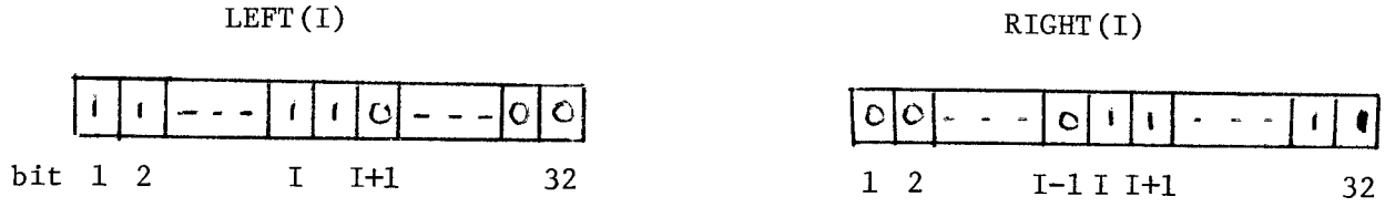
Fig. 3. LOGICAL*4 words LEFT(I) and RIGHT(I). Obviously 32 of each have to be defined.
