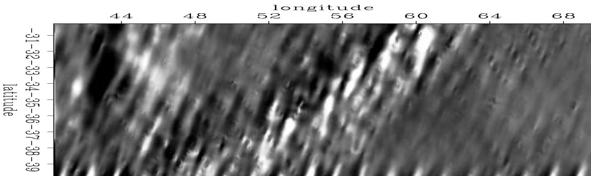
Figure 5: Model, regularized by PEF, created from southern sparsely sampled data, EW roughened by gradient. lomask1-allpef [ER]
