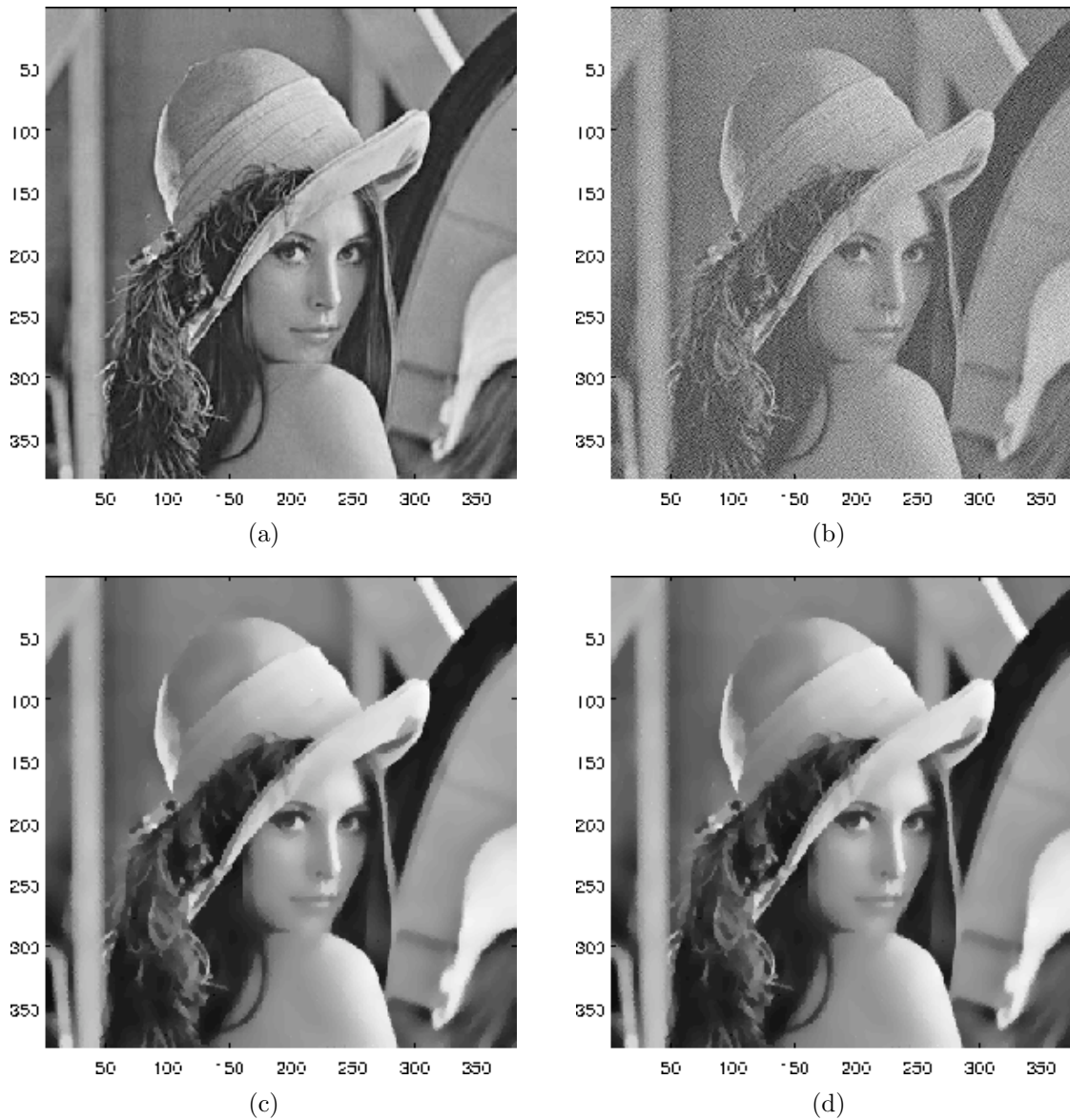
Figure B.1: (a) Clean image [NR]; (b) Noisy image contaminated with Gaussian noise with \sigma = 15\% of maximum amplitude [CR]; (c) Image denoised using Algorithm 4 with \alpha = 10 , \lambda = 1 and memory size m = 50 [CR]; (d) Image denoised using Algorithm 5 with \alpha = 10 , \lambda = 1 , N_c = 1 [CR]. ccd/. X1trueimg,X1noisyimg,X1ccd,X1rcg
