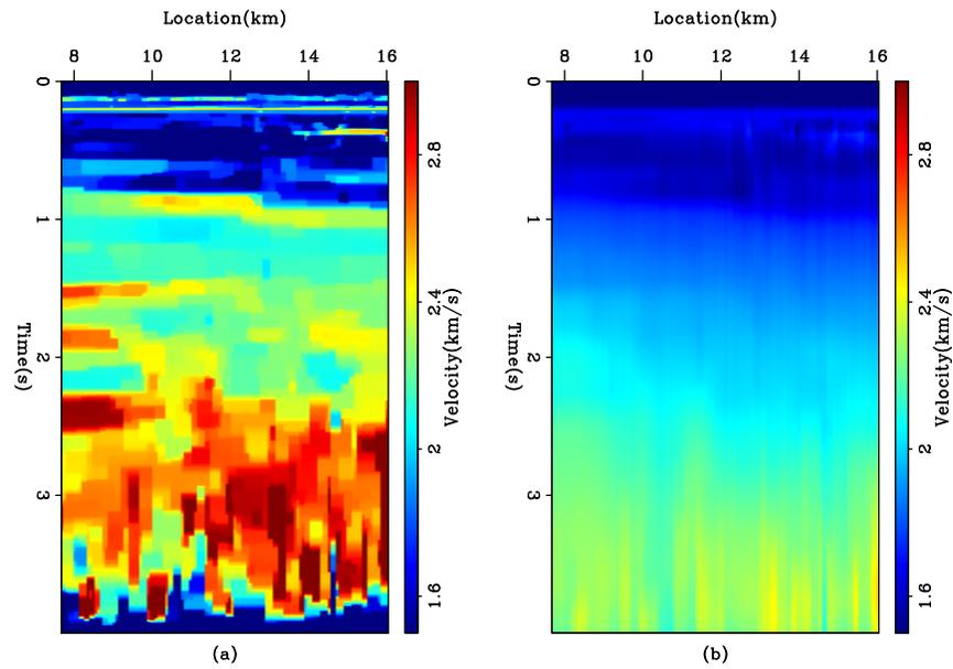
Figure 8: The WG dataset. (a) The interval velocity estimated by using the first derivative operator in two directions as a regularization in the hybrid norm. (b) The reconstructed RMS velocity. [ER]
