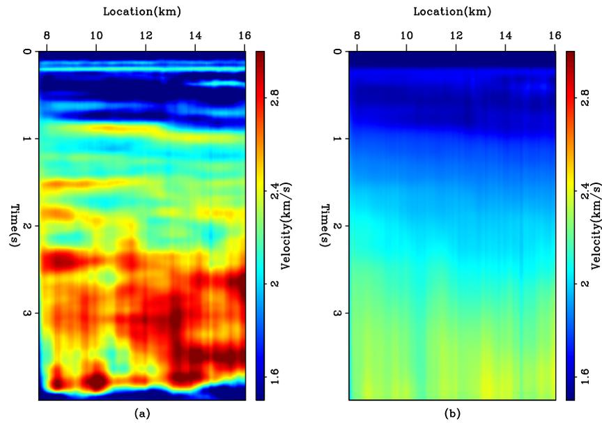
Figure 5: The WG dataset. (a) The interval velocity estimated by using the helix derivative operator as a regularization in the  $L_2$  norm. (b) The reconstructed RMS velocity. [ER]
