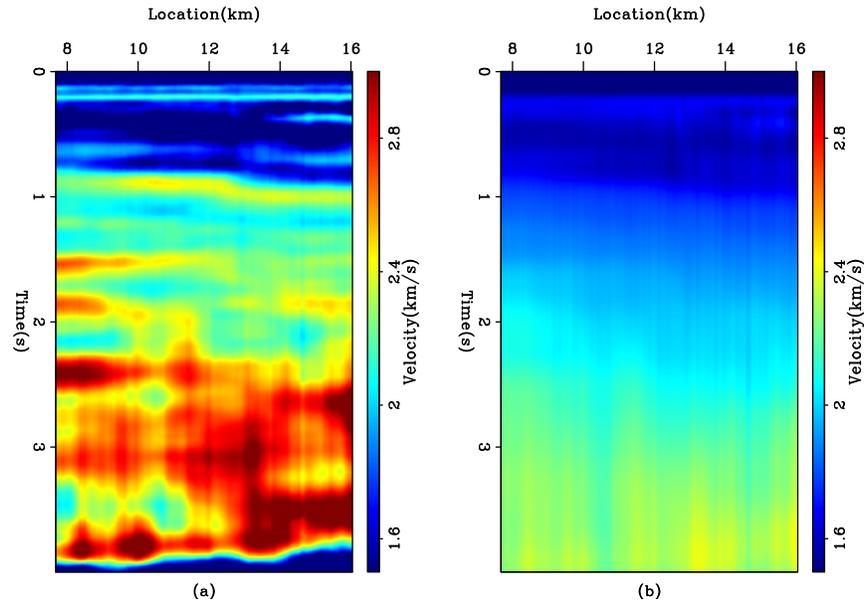
Figure 7: The WG dataset. (a) The interval velocity estimated by using the first derivative operator in two directions as a regularization in the  $L_2$  norm. (b) The reconstructed RMS velocity. [ER]
