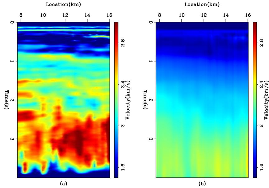
Figure 4: The WG dataset. (a) The interval velocity estimated by using the Laplacian operator as a regularization in the hybrid norm. (b) The reconstructed RMS velocity. [ER]
