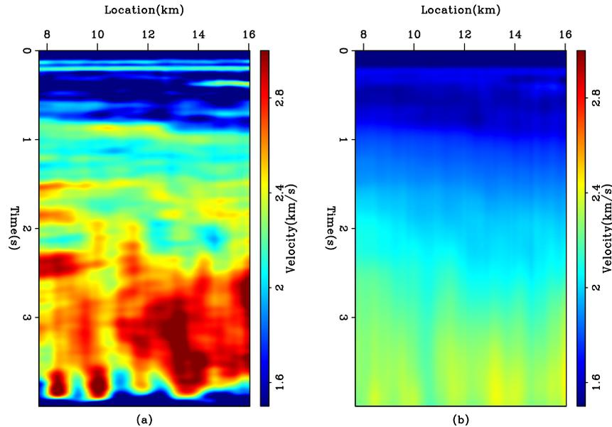
Figure 3: The WG dataset. (a) The interval velocity estimated by using the Laplacian operator as a regularization in the  $L_2$  norm. (b) The reconstructed RMS velocity. [ER]
