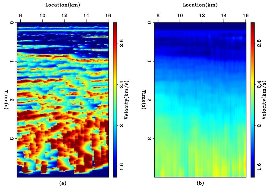
Figure 6: The WG dataset. (a) The interval velocity estimated by using the helix derivative operator as a regularization in the hybrid norm. (b) The reconstructed RMS velocity. [ER]
