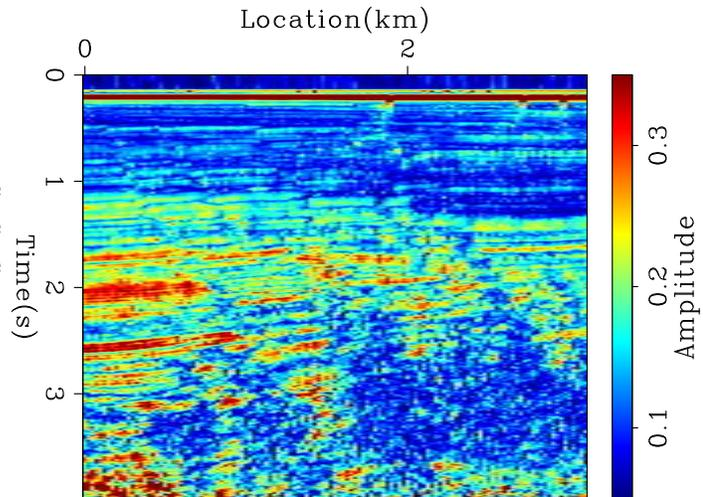
Figure 2: The strength of the picks in the velocity scan of the WG dataset, which is used as the weight before dividing by time. [ER]
