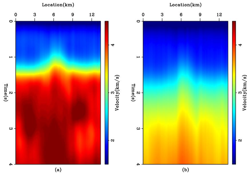
Figure 13: The ELF dataset. (a) The interval velocity estimated by using the first derivative operator in two directions as a regularization in the  $L2$  norm. (b) The reconstructed RMS velocity. [ER]
