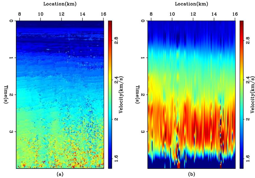
Figure 1: The WG dataset. (a) The input RMS velocity, which is automatically picked from the CMP gathers. (b) The interval velocity by direct dix conversion. [ER]
