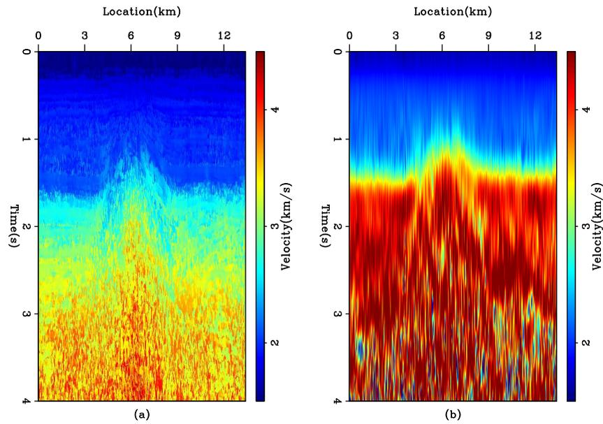
Figure 11: The ELF dataset. (a) The input RMS velocity which is automatically picked from the CMP gathers. (b) The interval velocity by direct Dix conversion. [ER]
