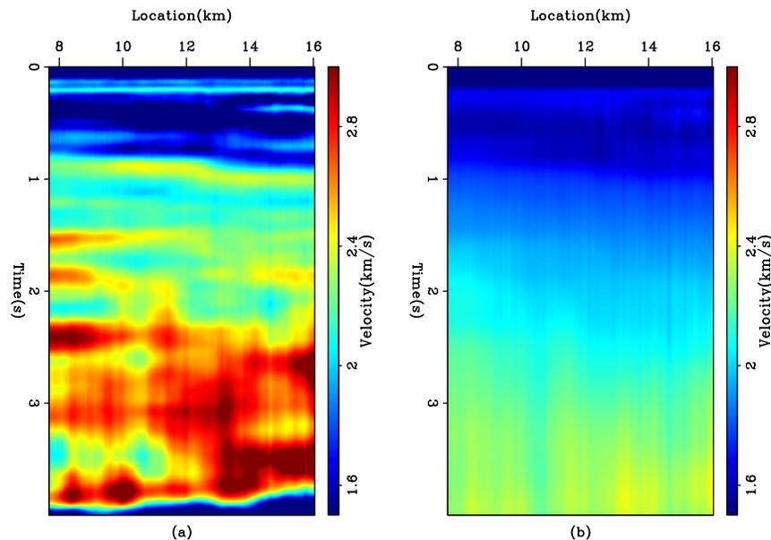
Figure 9: The WG dataset. (a) The interval velocity resulted by using the first derivative operator in four directions as a regularization in the  $L_2$  norm. (b) The reconstructed RMS velocity. [ER]
