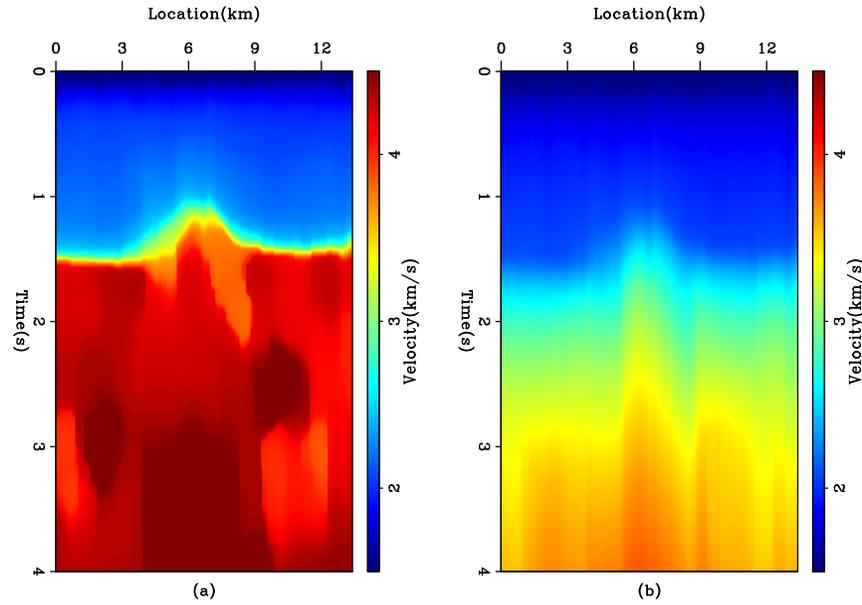
Figure 16: The ELF dataset. (a) The interval velocity estimated by using the first derivative operator in four directions as a regularization in the hybrid norm. (b) The reconstructed RMS velocity. [ER]
