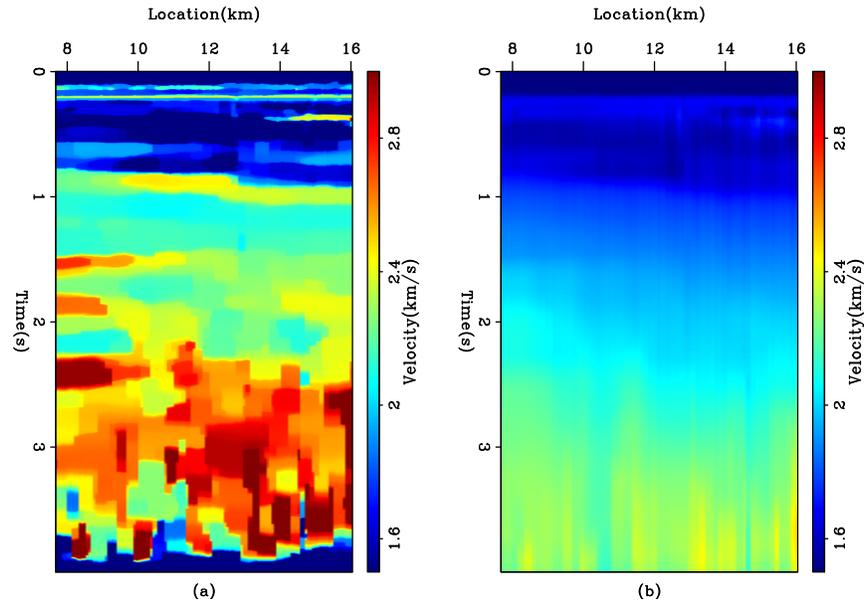
Figure 10: The WG dataset. (a) The interval velocity resulted by using the first derivative operator in four directions as a regularization in the hybrid norm. (b) The reconstructed RMS velocity. [ER]
