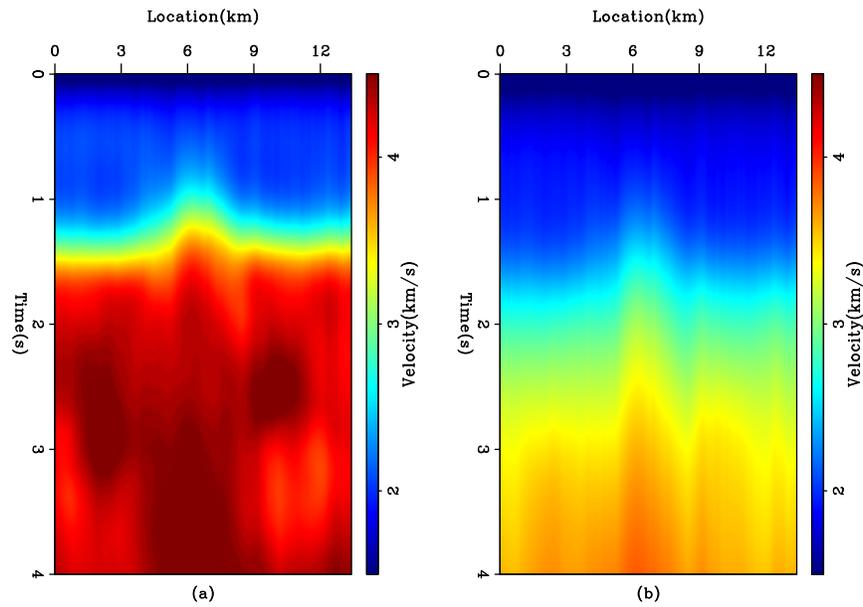
Figure 15: The ELF dataset. (a) The interval velocity estimated by using the first derivative operator in four directions as a regularization in the  $L_2$  norm. (b) The reconstructed RMS velocity. [ER]
