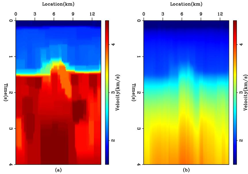
Figure 14: The ELF dataset. (a) The interval velocity estimated by using the first derivative operator in two directions as a regularization in the hybrid norm. (b) The reconstructed RMS velocity. [ER]
