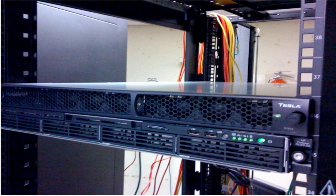
Figure 2: Rack mount view of the SEP Tesla system. At the top is the S1070 1U 4xGPU GPGPU Computing Appliance. Below is the HP ProLiant Xeon 64 bit, 8 core (2xSMP, 4xCMP) system, tesla0.stanford.edu which runs the host operating system. [NR]
