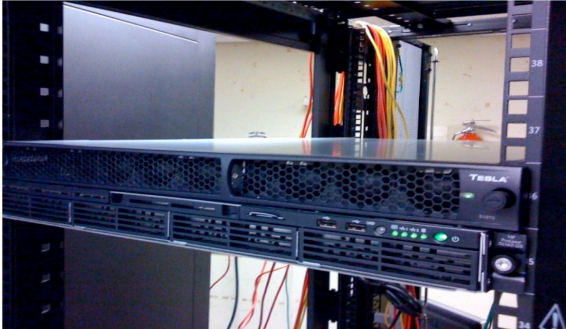
Figure 2: Rack mount view of the SEP Tesla system. At the top is the S1070 1U 4xGPU GPGPU Computing Appliance. Below is the HP ProLiant Xeon 64 bit, 8 core (2xSMP, 4xCMP) system, tesla0.stanford.edu which runs the host operating system. [NR] nwmoussa1/.teslaRackMountPhoto
