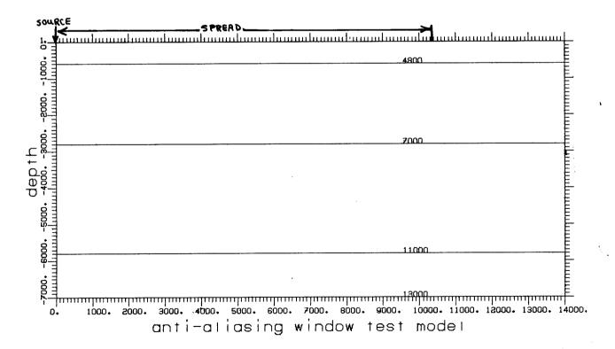
Figure 1.—Model 1: A water layer over sediments. The source and geophone locations are drawn in. The spread consisted of 48 geophones with a spacing of 220 feet.
