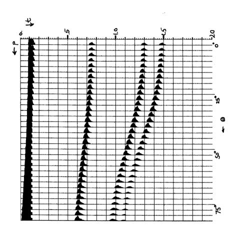
these gathers,  $P = \sin\theta/14000$ . Note the non-elliptical shape of the gather, this is due to Snell's The same field geometry was used to generate a common shot gather. The P-gather on the left was Figure 4.—The water layer of Model 1 was replaced by a 14000 ft/sec permafrost layer, computed with the anti-aliasing window and shows a great improvement over that in the right. law effects.
