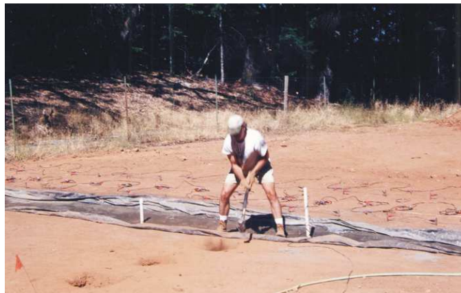
Figure 2.9: Data acquisition prior to construction of second trench, using “fan” geometry. Source point in this photo is one meter from one side of the trench, and receiver line is one meter from the opposite side of the trench. Shooter is standing in the trench, with PVC piezometers on either side of him that are used to measure water level in the trench. field-steve2 [NR]
