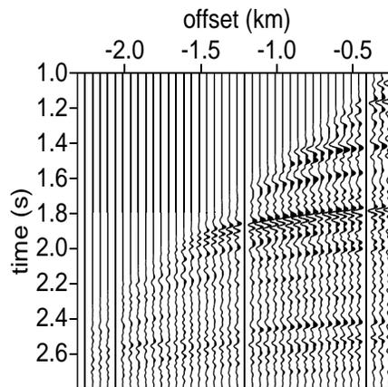
Strong surface related multiple energy is characteristic of this region. The main pre-processing steps were hyperbolic Radon filtering and bandpass filtering. The Radon filter suppressed but did not entirely remove coherent noise: it seemed reasonable to hope that primary energy dominates the filtered data, as is required by the dual regularization strategy. The bandpass filter ensured that the data were not spatially aliased, so that the differential semblance could be computed accurately.
