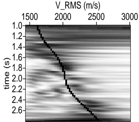
Figure 3: Image gather (= NMO corrected CMP) using  $V_{RMS}$  from velocity inversion with  $\sigma = 0.0$ . Note residual curvature in all events. `bill2-siginvdata0` [NR]
