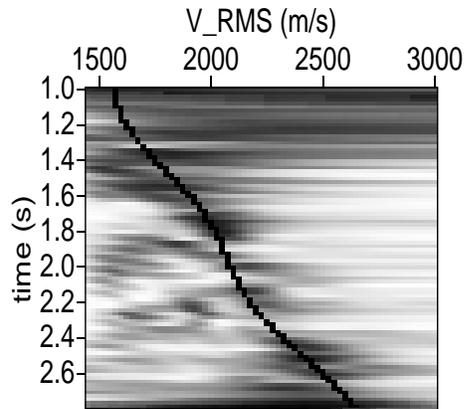
Figure 5: Image gather (= NMO corrected CMP) using  $V_{\text{RMS}}$  from velocity inversion with  $\sigma = 0.5$ . Primary reflections are essentially flat. `bill2-siginvdata5` [NR]
