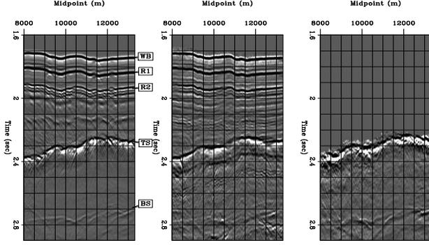
Figure 2: 2-D GoM imaging and stack. Left: Raw data. Center and right: Seabed (WB) and top of salt (TS) peglegs.
