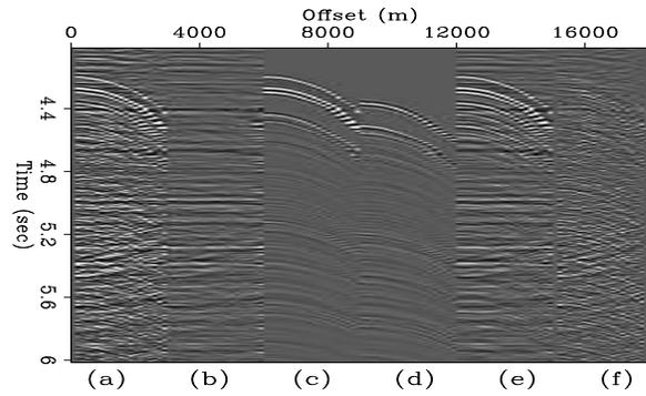
Figure 9: LSJIMP results on individual midpoint location (CMP<sub>x</sub>=100, CMP<sub>y</sub>=4). All panels NMO'ed, with  $t^2$  gain.
