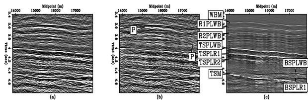
Figure 5: Zoom (CMP 13850-17850 m) of 2-D GoM stacked section before and after LSJIMP, with  $t^2$  gain. (a) Raw data; (b) Estimated primaries ( $m_0$ ); (c) Difference. Events labeled as in Figure 3. Subsalt primary labeled "P".
