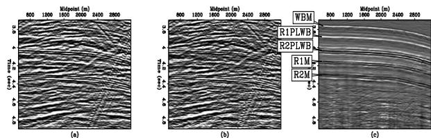
Figure 4: Zoom (CMP 500-3200 m) of 2-D GoM stack before and after LSJIMP, with  $t^2$  gain. (a) Raw data; (b) Estimated primaries ( $m_0$ ); (c) Difference. Events labeled as in Figure 3.
