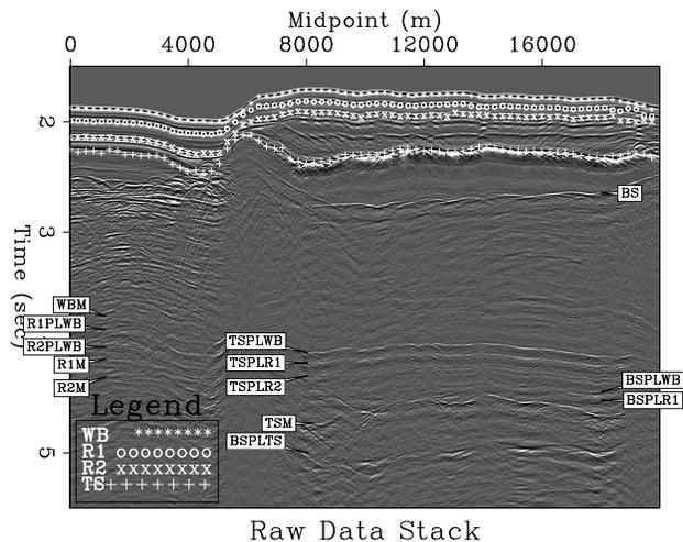
Figure 3: Stacked 2-D GoM data, after  $t^2$  gain. Picks denote the four multiple generators (seabed - WB, R1, R2, and top of salt - TS). Naming convention for pure multiples: (*reflector*)M and for pegleg multiples: (*target*)PL(*multiple generator*), e.g., BSPLWB.
