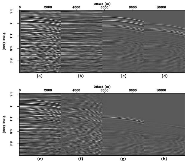
Figure 6: 2-D GoM CMP 55 (1440 m) before and after LSJIMP. Panels defined in text. All panels NMO'ed, windowed from 3.5 to 5.5 seconds, and gained with  $t^2$ .
