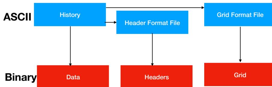
Figure 1: The six files representing a SEP3D dataset. The arrows represent which files point to other files.
