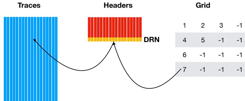
Figure 2: How to read a trace from a SEP3D dataset. First read the grid to get a pointer into the headers. Look in the headers for DRN key, which provides the location within in the traces.
