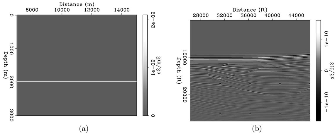
Figure 2: Reflectivity models in slowness squared. a) Flat model; b) Sigsbee model. [ER]
