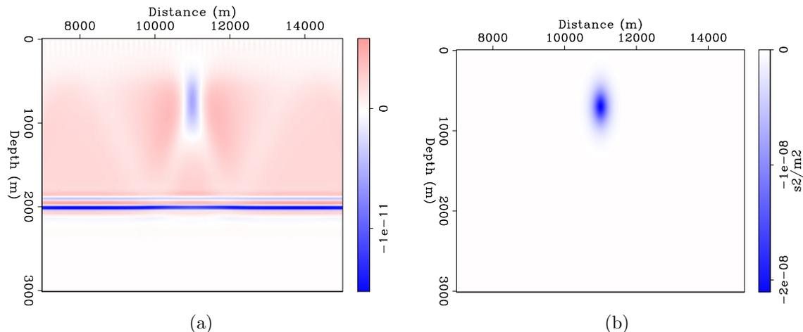
Figure 5: Flat model: a) First gradient of the nonlinear image power maximization term; b) True perturbation of the background in slowness squared. [CR]
