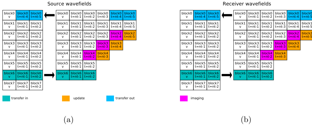
Figure 3: Pipeline algorithm for computing the gradients: (a) source wavefield pipeline and (b) receiver wavefield pipeline. [NR]
