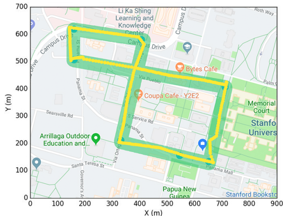
Figure 9: While there still remains uncertainty in the mapping process, the Markov decision process generates approximate mappings at low cost (yellow), since human input is limited to defining the guiding path (green). Background image courtesy of Google Maps. [CR]
