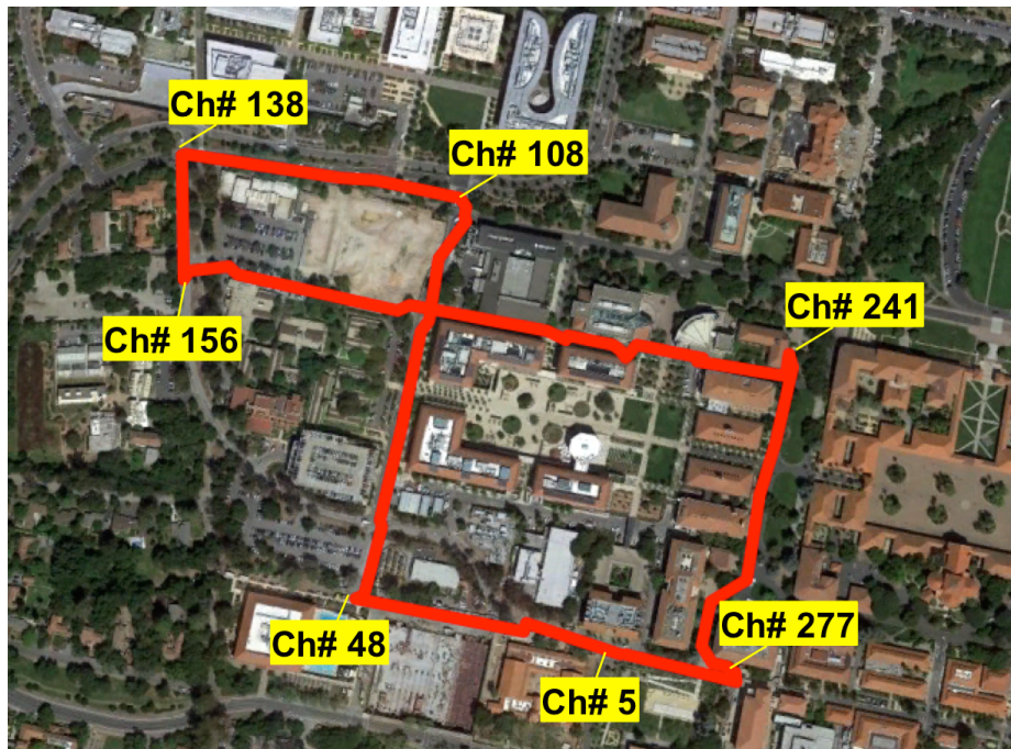
Figure 1: Map showing the path of SDASA-1 with the location of the corner points of the array marked and labeled with the corresponding channel numbers. [NR]
