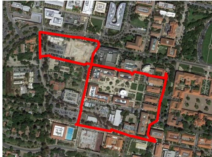
Figure 1: The fiber optic cable (red line) is deployed under Stanford campus in the telecommunication infrastructure tunnels. It forms a North-East and a South-West loop. [NR]
