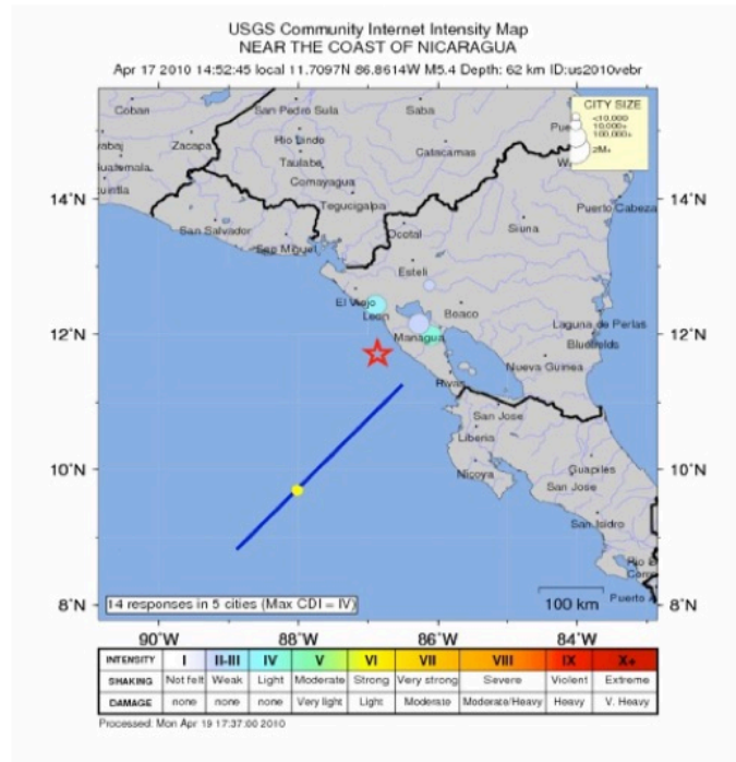
Figure 3: USGS report pertaining to the earthquake (indicated by the red star) that occurred during the SERPENT EM survey. The blue line indicates the EM ocean-bottom node line, where the yellow dot is the position of the composite sensor which had a three-component geophone in addition to the EM sensors. [NR] ohad1/. M54EQ
